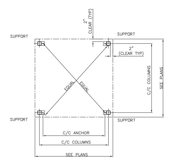
NOTE: Required clearance for landing edges in diagram above. Layout column locations using a chalk line. Refer to drawings provided with your order. Using hammer drill with 1/2" concrete bit, drill holes 4" deep and remove all debris before placing columns and inserting anchors.
