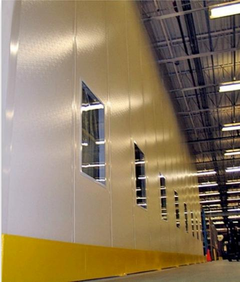
Constructed of single piece, 3" to 4" thick, steel-faced insulated panels up to 30 feet high, our Hi Wall™ system is custom-installed around existing pipes, joists and structures. This panel systems features 26 gage, G90 hot-dip galvanized facings with baked-on acrylic enamel, providing you with unmatched strength and durability. It is also Class A fire rated and utilizes ThermalCore™ EPS insulation, and to suit your needs, optional urethane insulation if higher R-values are required.
